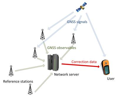
Figure 1. Structure of a ground-based augmentation network
